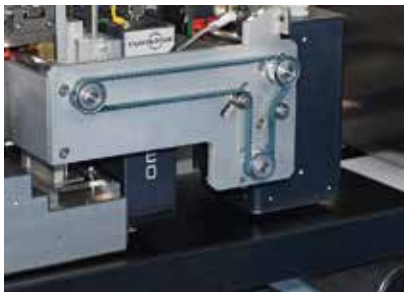
The centerpiece of DIGILINE Label – Offline is the contact-free OMEGA DoD UV inkjet printer. It guarantees even at high production speeds a brilliant and durable printing quality. The optional automatic cleaning station ensures full availability.
