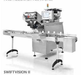
The Swiftvision counter range can be configured for any product or container requirement. Count speed and accuracy are optimized through the unique auto balanced feeding system, which prevents surges and ensures a constant flow of the product to the count head, independent of the hopper level. The counters are available in Single, Twin and Duplex versions.
